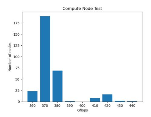
InfiniBand in some compute nodes is not stable. We had to pick out the bad nodes.
