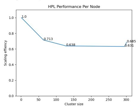
As the number of nodes increases, the scaling efficiency becomes progressively lower, and the rate of decrease tapers off to about 0.63 at 300 nodes. in our experiments, an unexpectedly high scaling efficiency occurs when used a specific number of nodes, such as 301. we believe this is related to the topological of the nodes (P, Q, NB).
